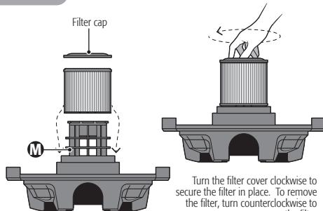
Turn the filter cover clockwise to secure the filter in place. To remove the filter, turn counterclockwise to remove the filter
