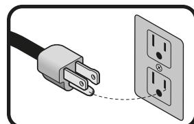
**⚠ CAUTION** When using an extension cord, verify the gauge is enough for the power that your product needs. A lower gauge cable will cause voltage drop in the line, resulting in power loss and overheating. The following table shows the right size to use depending on cord's length and the ampere capability shown on the tool's nameplate. When in doubt use the next higher gauge.
