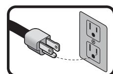
**WARNING** Do not modify the plug supplied. If the plug cannot be fitted to the socket, have a qualified electrician to install the suitable socket.
