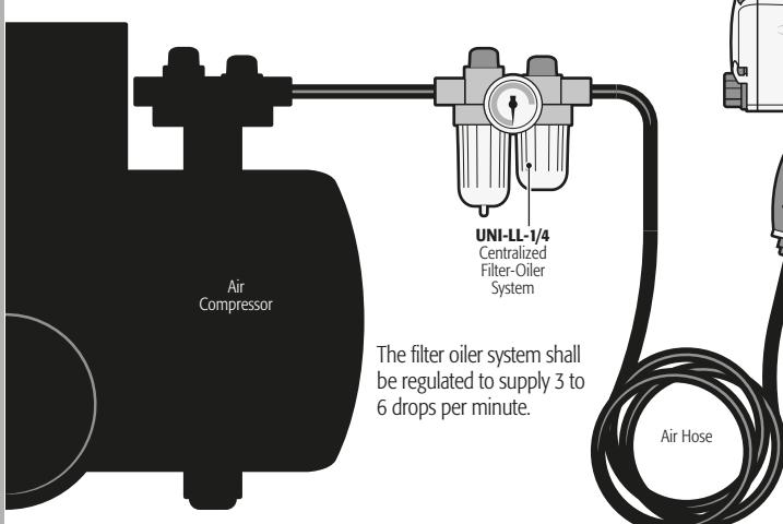
The filter oiler system shall be regulated to supply 3 to 6 drops per minute.
