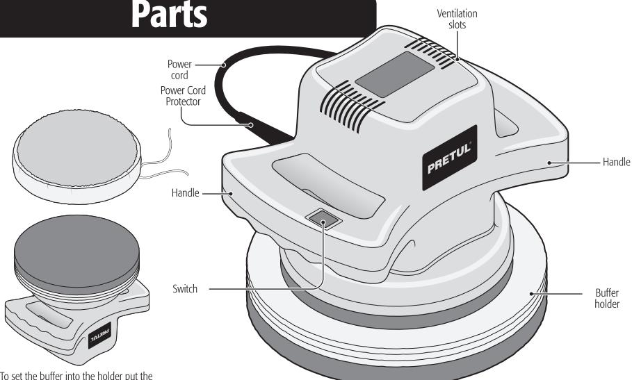
To set the buffer into the holder put the polisher upwards. Untie the buffer string and wrap the holder with the buffer. Turn around the polisher back. Tighten and make a knot with the string to fix the buffer in place.
