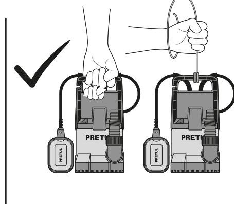
It is recommended to tie a rope to the carrying handle to lift the pump.
