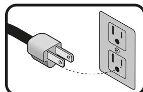
**⚠ WARNING** When using an extension cable, verify the gauge is enough for the power that your product needs. A lower gauge cable will cause voltage drop in the line, resulting in power loss and overheating. The following table shows the right size to use depending on cable's length and the ampere capability shown in the tool's nameplate. When in doubt use the next higher gauge.
