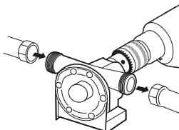
The drill pump will work when you start the hand drill, please confirm whether the steering of the hand drill is consistent with that of the drill pump.
