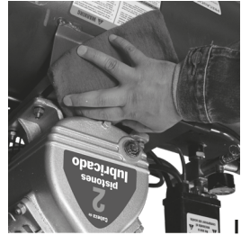
I CLEANSING: Keep the inside and outside of the compressor clean. Replace oil regularly and keep all the external surfaces clean. A clean inner side guarantees good mechanical efficiency and a clean exterior allows circulating air heat to dissipate efficiently. (See figure I).
