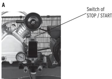
**NOTE:** Before starting the compressor any compressed air remaining above the piston and in the feeding pipe shall be discharged. Press the pressure switch button and lift it again into the "1" (ON) position. The motor will start immediately.
