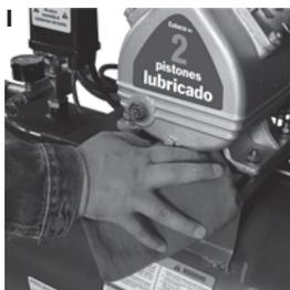
**CLEANSING:** Keep the inside and outside of the compressor clean. Replace oil regularly and keep all the external surfaces clean. A clean inner side guarantees good mechanical efficiency and a clean exterior allows circulating air heat to dissipate efficiently. (See figure I).
