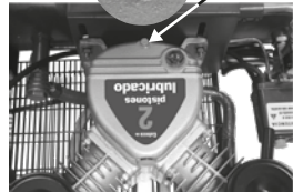
H EVERY FOUR MONTHS OR AFTER 500 HOURS USE OIL: Drain oil and refill up to the right level using SAE-30 motor oil. (See figure h)
