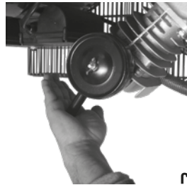
J SUCTION ACTION: Put your hand lightly onto the filter admission orifices. You will clearly hear the air suction. A deficient suction suggests the air filter is blocked or the admission valves are damaged. (See figure j).
