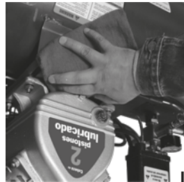
I CLEANING: Keep the inside and outside of the compressor clean. Replace oil regularly and keep all the external surfaces clean. A clean inner side guarantees good mechanical efficiency and a clean exterior allows circulating air heat to dissipate efficiently. (See figure i).
