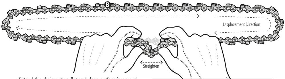
• Extend the chain onto a flat and clean surface in an oval shape, together with the chain bar and straighten any twisted link. The cutting sprockets shall face the chain displacement direction, otherwise reverse the chain position.
