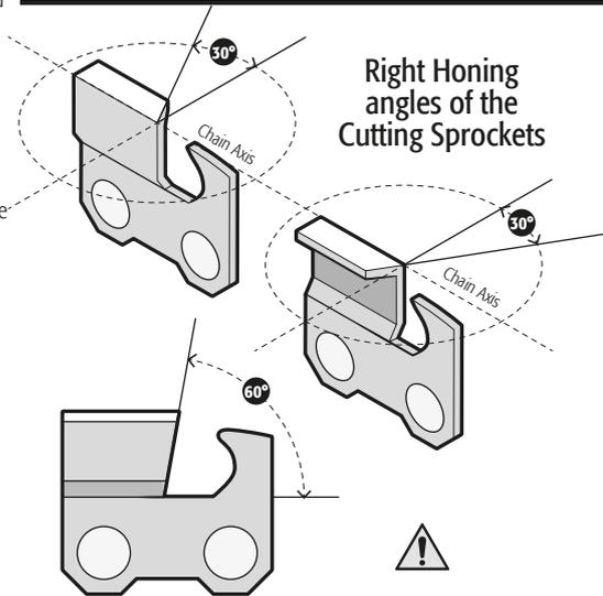
**WARNING** Any other angle different to the specified lessens the cut quality, damages the motor, the bar and chain and increases the risk of a violent kickback.
