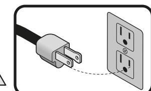
**⚠ WARNING** When using an extension cable, verify the gauge is enough for the power that your product needs. A lower gauge cable will cause voltage drop in the line, resulting in power loss and overheating. The following table shows the right size to use depending on cable's length and the ampere capability shown in the tool's nameplate. When in doubt use the next higher gauge.
