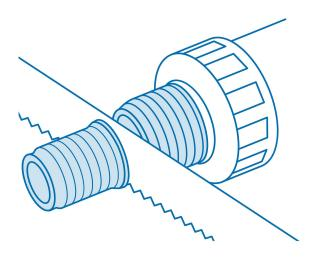
Para conectar a 1" NPT, cortar tramo 3/4" NPT
